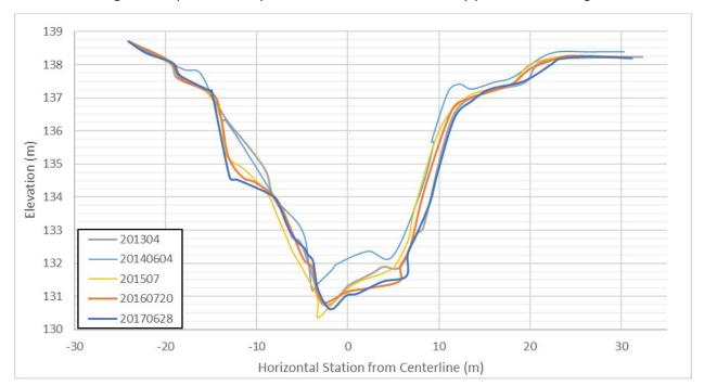
Figure 1. Aquilla Creek upstream cross-section for survey years 2013 through 2017
